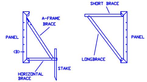
NOTE: HORIZONTAL BRACE CAN BE FASTENED TO BOLT HOLE (B) TO EASE PLUMBING INSTALLATION.
